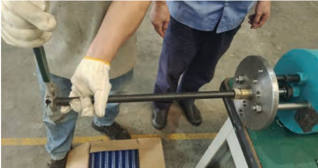
Install the screw, screw one end of the screw screw completely screw into the inner screw of the piston rod, and then press the screw sleeve completely into the step hole of the pressure plate part of custom tool.
