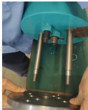
Install the pressure plate part of special custom tool, then attach the special Allen wrench to the piston rod nut.
