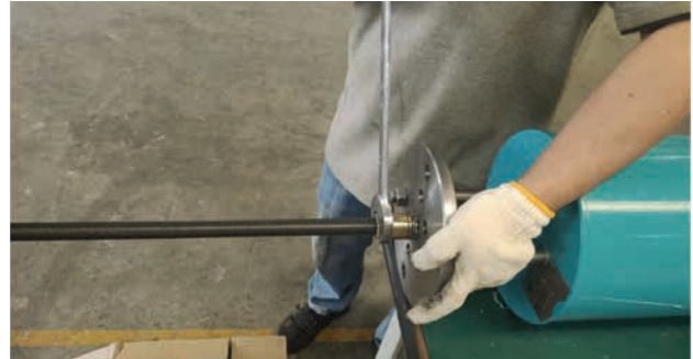
Install the screw, screw one end of the screw screw completely screw into the inner screw of the piston rod, and then press the screw sleeve completely into the step hole of the pressure plate part of custom tool.
