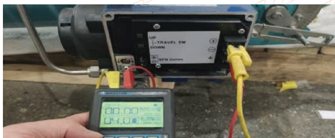
The positioner is connected to a 4-20mA signal source, and controls the actuator through the positioner to check the operation of the actuator.
