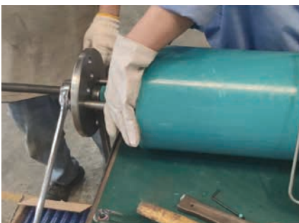
Continue to turn the screw sleeve clockwise until the end cover and the cylinder body contact surface are completely overlapped.
