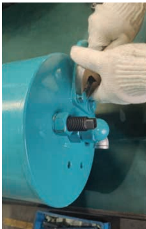
Removing the ring, lock screw, piston rod nut and weather cap.
