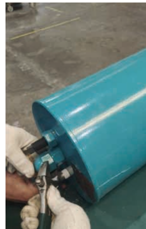
Removing the ring, lock screw, piston rod nut and weather cap.
