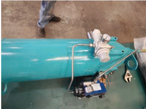
Turn off the air source so that the actuator is fully closed.
