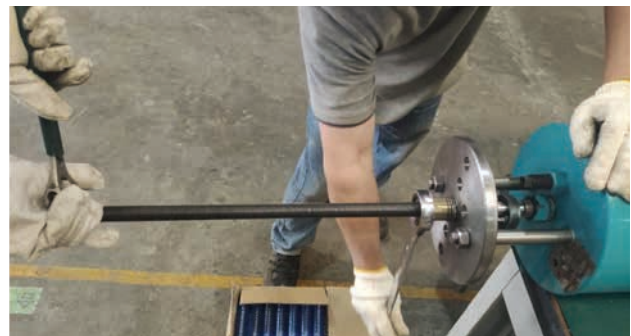
Use a wrench to turn the screw sleeve counterclockwise so that the end cap is gradually withdrawn.
