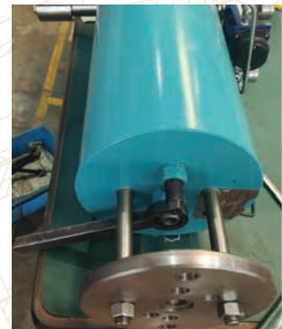
Install the pressure plate part of special custom tool, then attach the special Allen wrench to the piston rod nut.
