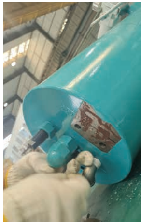
Removing the ring, lock screw, piston rod nut and weather cap.
