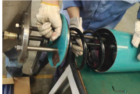
Install tooling, connect screw and piston rod.
