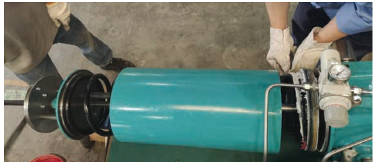
Continue to turn the screw sleeve clockwise, and the other person needs to constantly adjust the spring position during this process to ensure that the spring and the piston are concentric at all times until the spring is compressed to the point that it is not affected by other forces and the piston is eccentric.
