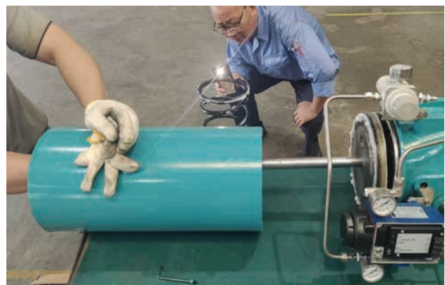
Take out the spring and cylinder block, check the cylinder parts, and replace or repair relevant parts.
