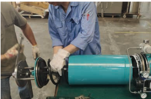
Turn the screw sleeve clockwise so that the spring is pressed against the end cover and piston face
